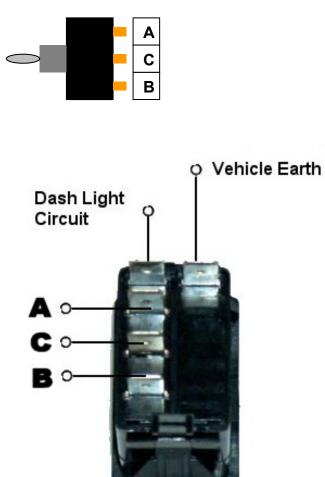
The letters A,C & B are shown for the corresponding terminals on each type of switch. If you would like the switch to light up with your other dash panel lights, then connect the top two terminals as shown.
