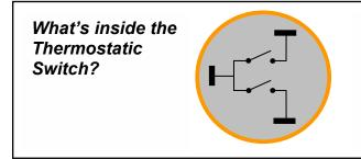
The 50091 switch just contains a pair of switches controlled by bi-metallic strips (which bend proportionally to the temperature). When the temp is high enough, the strip closes the contacts, completing that circuit.
